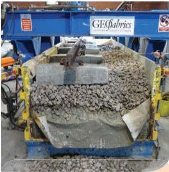
Failed pumping test using standard geotextile separator.
