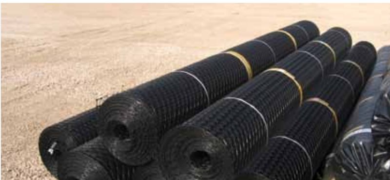
Reinforcing weak soil in Ashbourne, Derbyshire
