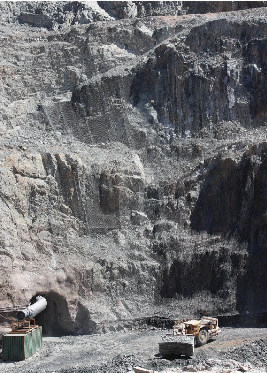
Portal protection – note the fly rock damage to the netting in a couple of locations caused by close proximity blasting. Unlike single twist (fencing type) mesh, the double twist technology ensures the mesh structure cannot unravel in these areas and tensile strength is maintained
