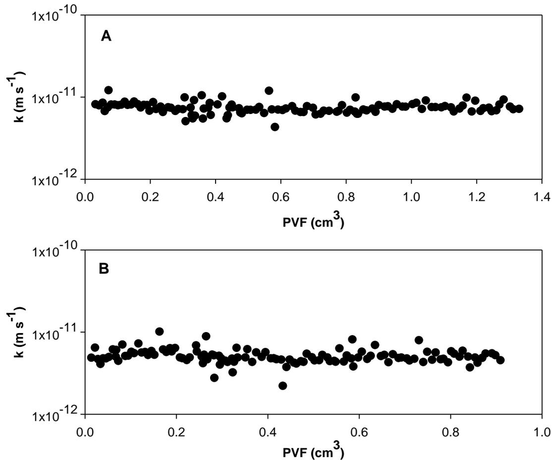
Figure 2. Saturated hydraulic conductivity ( $k_{\text{Triaxial}}$ ) of ABM2 in 20% saline-sodic brine; A) non pre-hydrated, B) pre-hydrated in deionised water.
