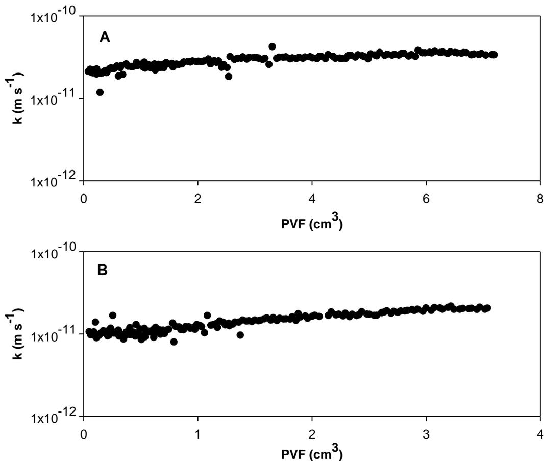
*Figure 1. Saturated hydraulic conductivity ( $k_{\text{triaxial}}$ ) of ABM2 in 2M NaCl; A) non pre-hydrated, B) pre-hydrated in deionised water.*
